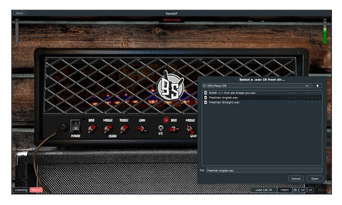
When pressed, a file choosing dialog opens up (the last used path is always stored to your convenience) to choose an IR audio file (in \*.wav format). You can switch from intern to extern IR via *intern/extern* button. The IR based cabinet emulation can also be switched off, to use your own *Impulse Response Player* (on/off-Button at the right lower corner).
