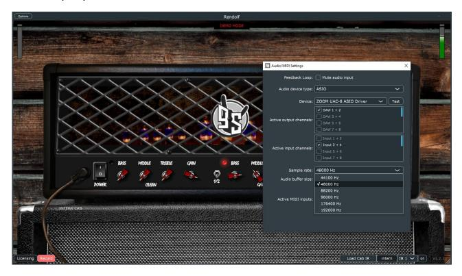
After that, please set the *sample rate* according to your needs. As rule of thumb: the higher the *sample rate* the better the sound quality of the plugin but the bigger the *audio buffer* size must be set in your audio interface settings to not introduce distortion artifacts, to fulfill the real-time constrains.
