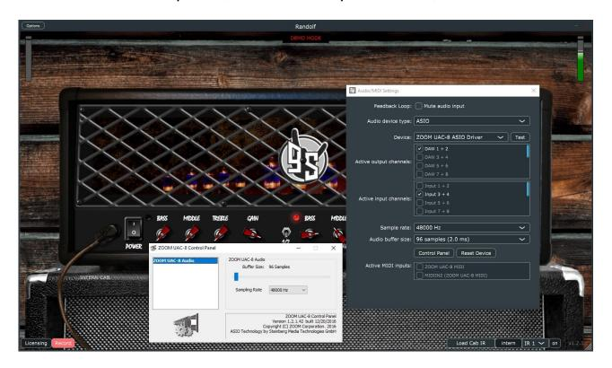
here you have to increase the *buffer size* of your audio device until no distortion artifacts are hearable on a chosen *sample rate*.
