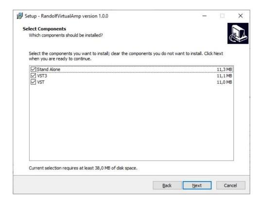
**Remark:** The VST3 Plugin will be installed in a standard folder on your system (usually: C:\Program Files\Common Files\VST3).
