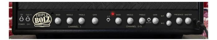
In between the parametric equalizer (EQ) and gain section knobs for each channel are located. IN between the EQ sections a toggle switch to change between CH2/3 is placed. Between the Treble and Gain knob a Boost knob is located to switch On/Off the Tube Screamer Boost (which is placed as usual
