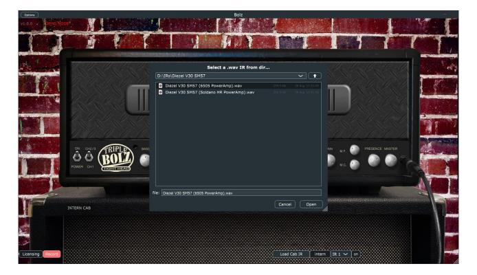
When pressed, a file choosing dialog opens up (the last used path is always stored to your convenience) to choose an IR audio file (in \*.wav format). You can switch from intern to extern IR via *intern/extern* button. The IR based cabinet emulation can also be switched off, to use your own *Impulse Response Player* (on/off-Button at the right lower corner).
